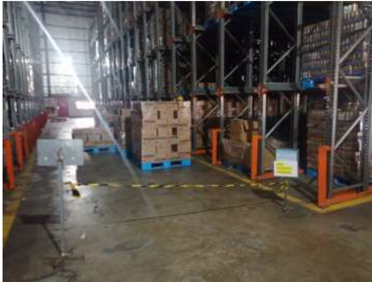
Plate 2.4: Blocked Passageways in the Warehouse
