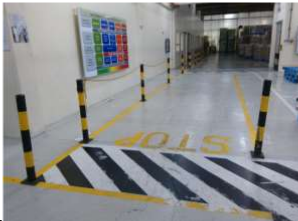
Plate 2.1: Prevention Risk of Collision between People and Moving Equipment
