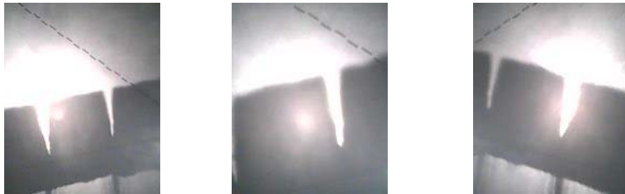
Figure 4.7: Effect of the number of passes on kerf widths for different materials
