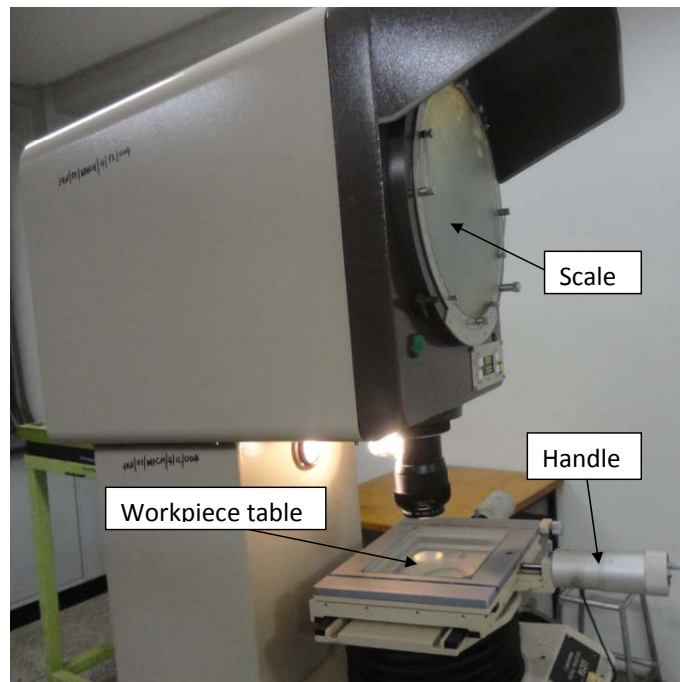
Figure 3.12: Taking of measurements using a Profile Projector
