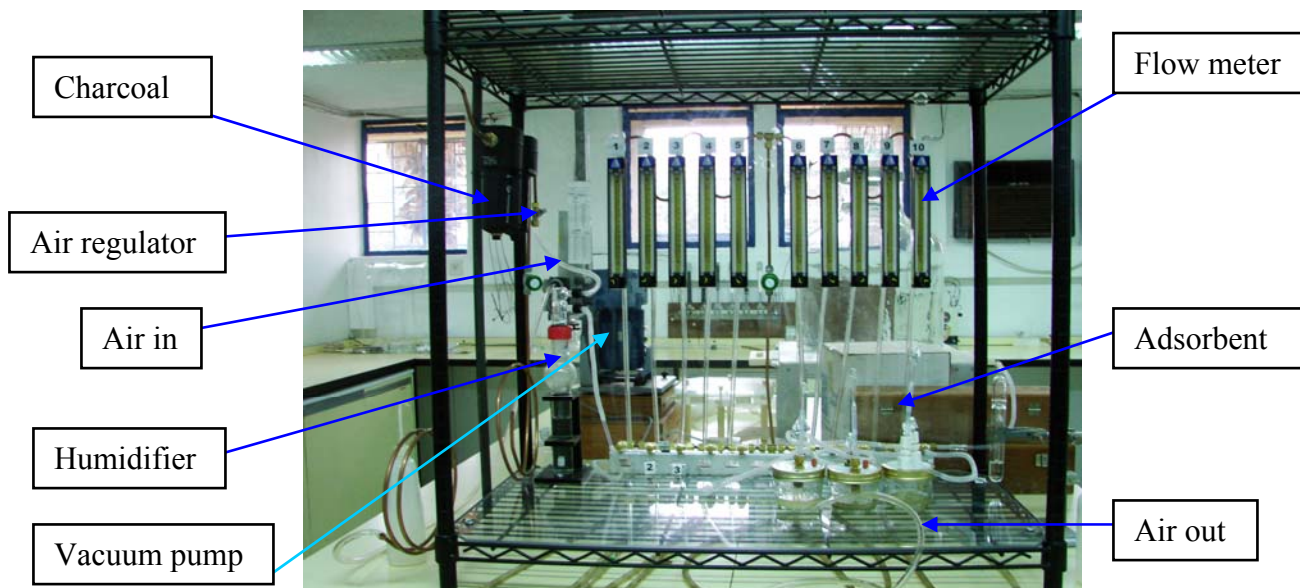
Plate 3.1. Dynamic volatile collection system.
