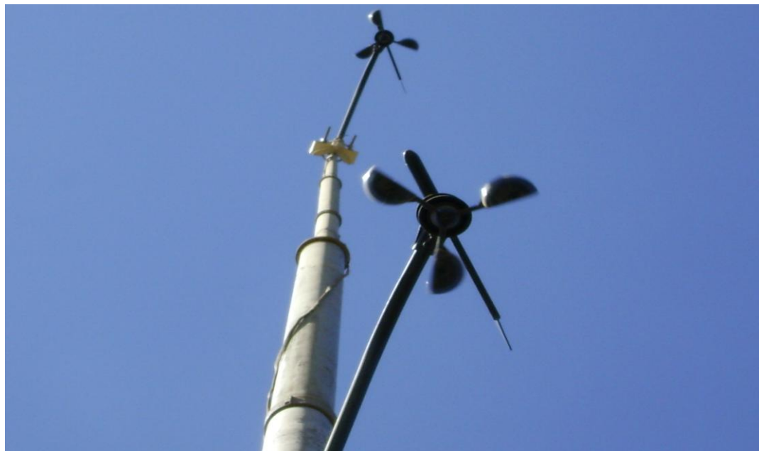
Plate 3: The wind sensors clamped on a mast
