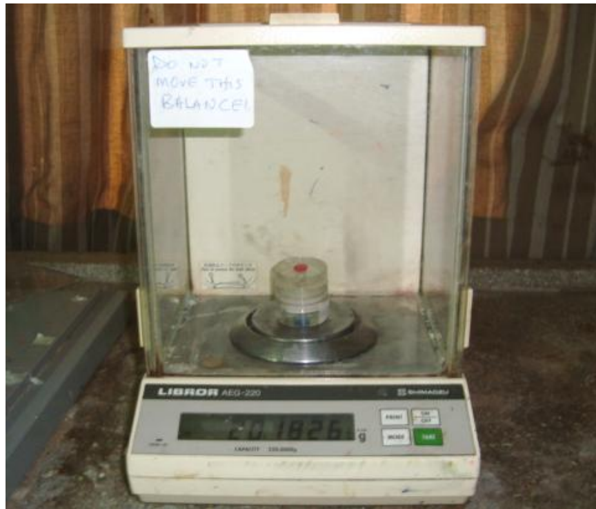
Plate 10 Pre and post sample weighing of dust sampling unit to determine the amounts of respirable dust collected
