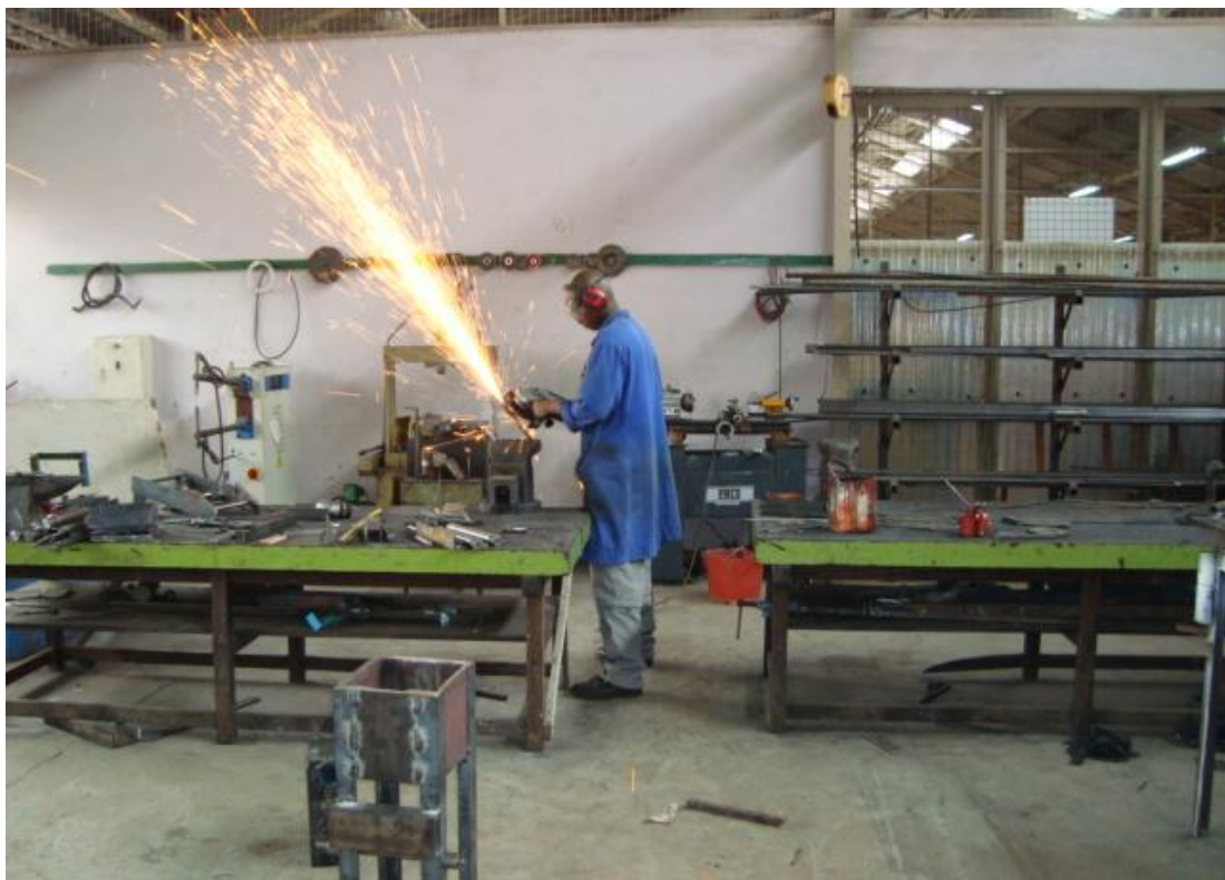
Plate 5 A typical noisy activity that provided noise sampling data in a high noise generation workplace
